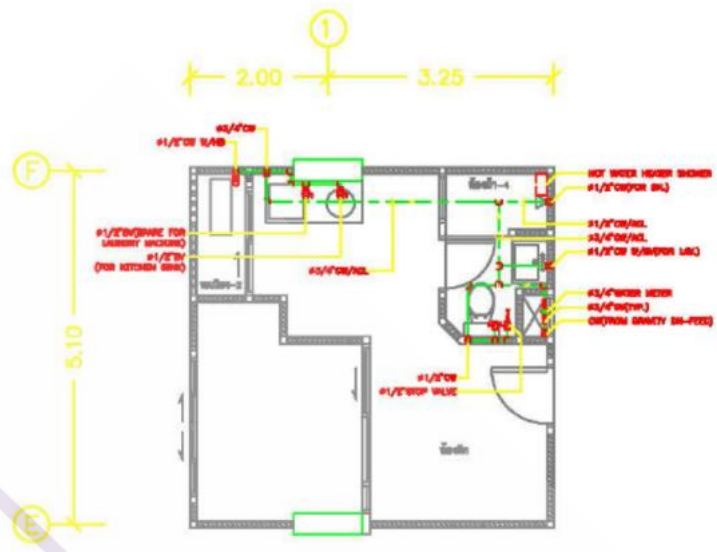
COLD WATER SYSTEM LAYOUT PLAN (SUPPLY FROM GRAVITY DIS-FEED) (2nd-4th. FLOOR)
