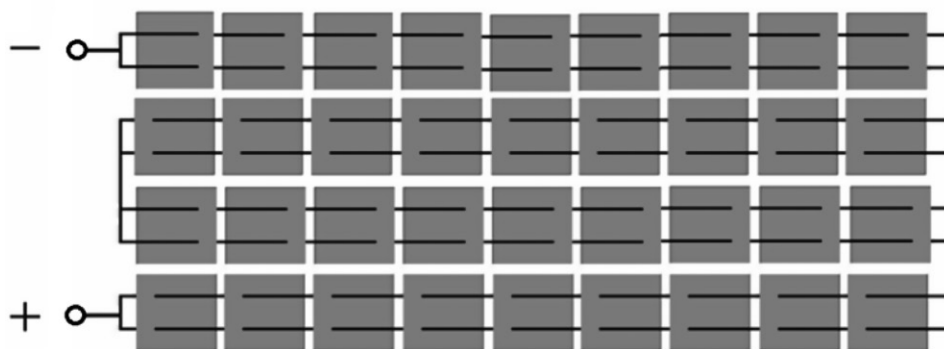
FIGURE 9.24 A common module configuration of 36 series-connected cells.
