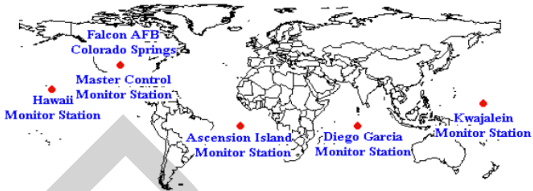
Global Positioning System (GPS) Master Control and Monitor Station Network
